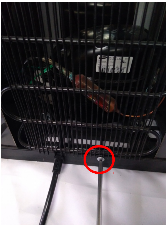
11- Reinstall the grid in the back of the cooler and screw the two screws on the top and the one at the bottom. Plug back your cooler and test it.
