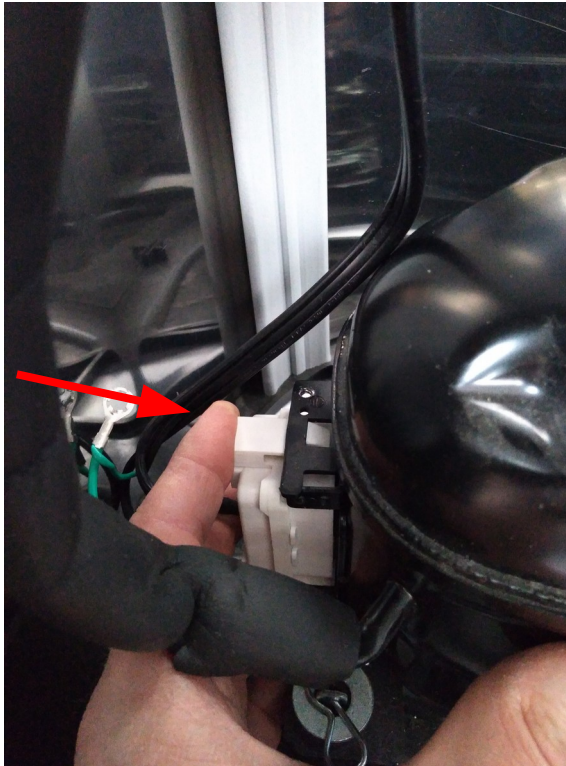
9- Push the new relay by hand to lock the upper tab and reinstall the two connectors on the relay.
