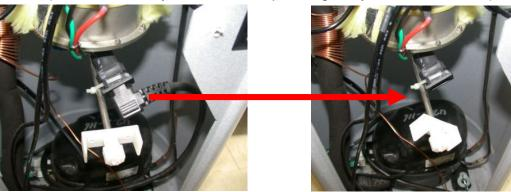
Step #6 Unplug the two wires of the ON/OFF switch
