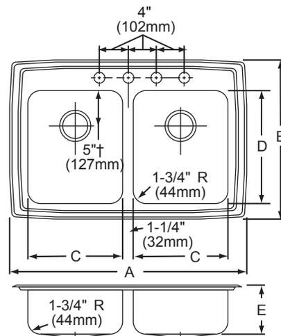
Model LRAD(Q) Series Off-Centered Drain
