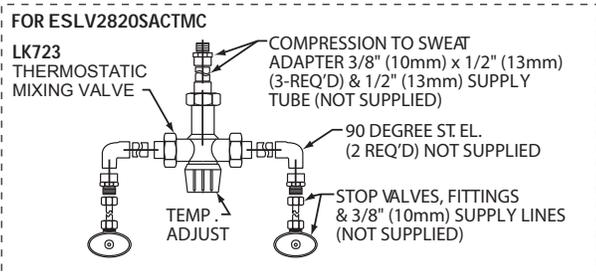
NOTE: USE TEFLON TAPE FOR ALL WATER CONNECTIONS. DO NOT USE PIPE DOPE.
