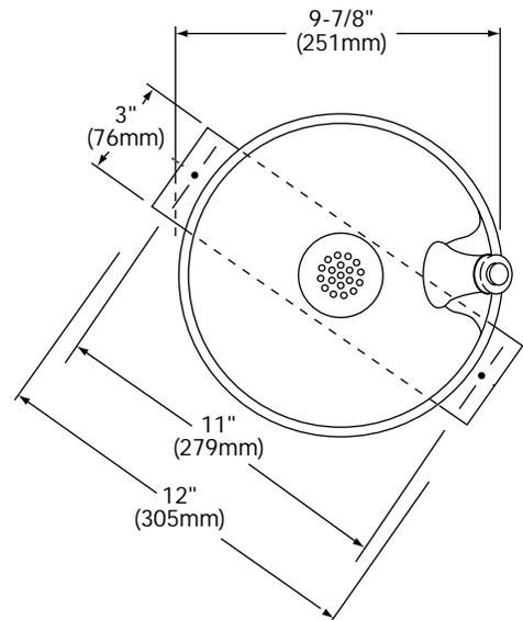
NOTE: ROUGH-IN DIMENSIONS MAY VARY 1/2" (13mm) PLUS OR MINUS. BUBBLER CAN BE MOUNTED ON RIGHT OR LEFT AS DESIRED.
