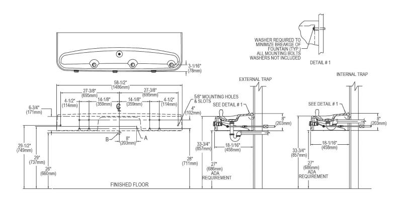
LEGEND A = 3/8" O.D. Unplated copper tube connect - shut off valve by others B = Water outlet 1-1/2" O.D. drain stub out from wall 1" (25mm)
