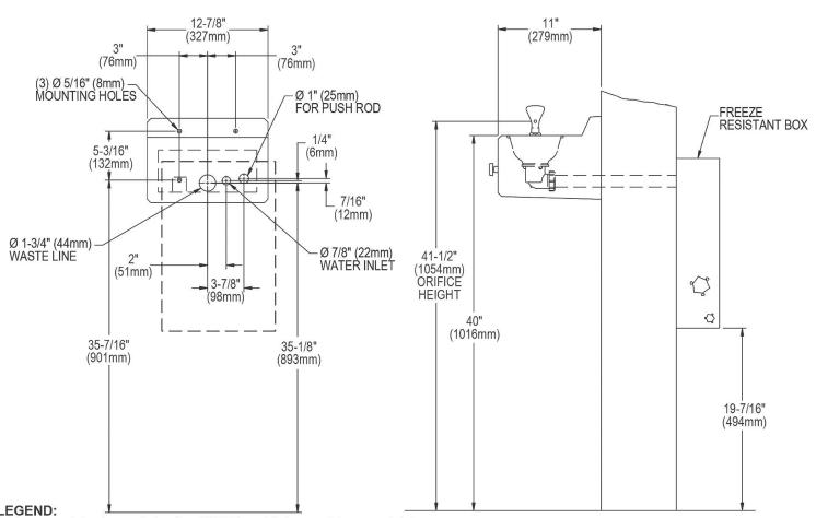
A: Recommended water supply location, 3/8" O.D. unplated copper tube connect stub 1-1/2" (38mm) out from wall shut off valve by others.
