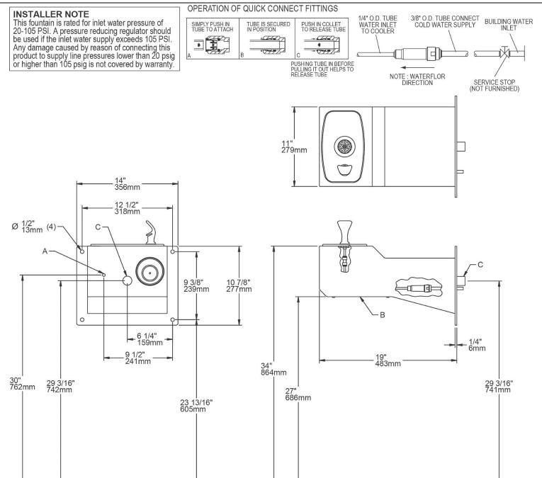
A = 3/8" (10mm) O.D. unplated copper tube connect - shut off valve by others.
