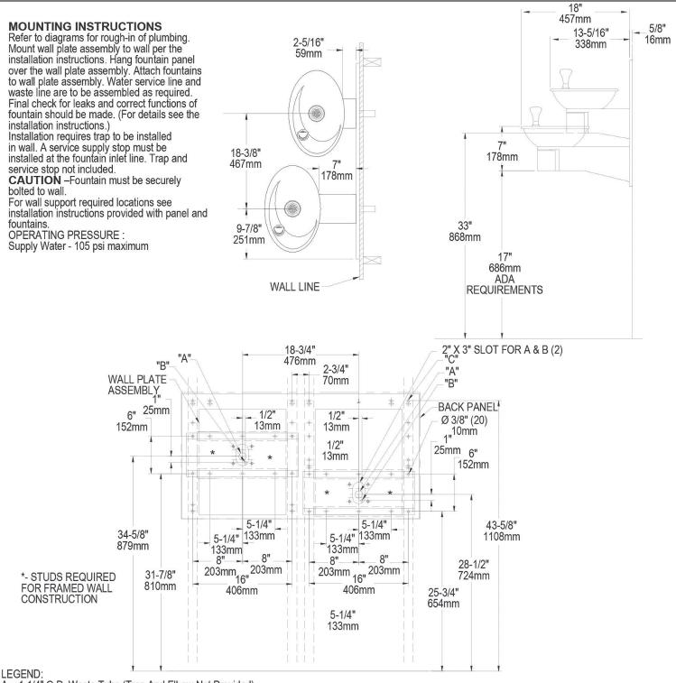
A = 1-1/4" O.D. Waste Tube (Trap And Elbow Not Provided) B = 3/8" O.D. Unplated Copper Tube Connect (Water Inlet) C = 1/4" DIA. (6mm) Holes For Mounting Plate To Wall
