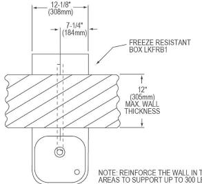
WARNING: The free-resistant box must be installed on an interior heated wall where the temperature does not drop below 50° F (10° C). The front of the box must have unobstructed air flow. Failure to maintain the interior wall temperature and the inside of the freeze resistant box above 50° F (10° C) can result in damage to the box which could result in unrestricted water flow.
