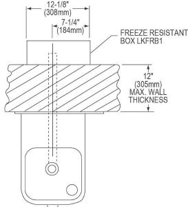
**WARNING:** The free-resistant box must be installed on an interior heated wall where the temperature does not drop below 50° F (10° C). The front of the box must have unobstructed air flow. Failure to maintain the interior wall temperature and the inside of the freeze resistant box above 50° F (10° C) can result in damage to the box which could result in unrestricted water flow
