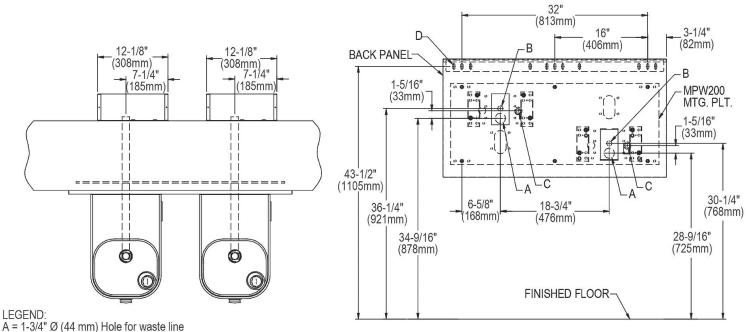
A = 1-3/4" Ø (44 mm) Hole for waste line B = 7/8" Ø (22 mm) Hole for water supply C = 7/8" Ø (22 mm) Hole for operating cable D = 1/4" Ø (6 mm) Hole for mounting plate to wall
