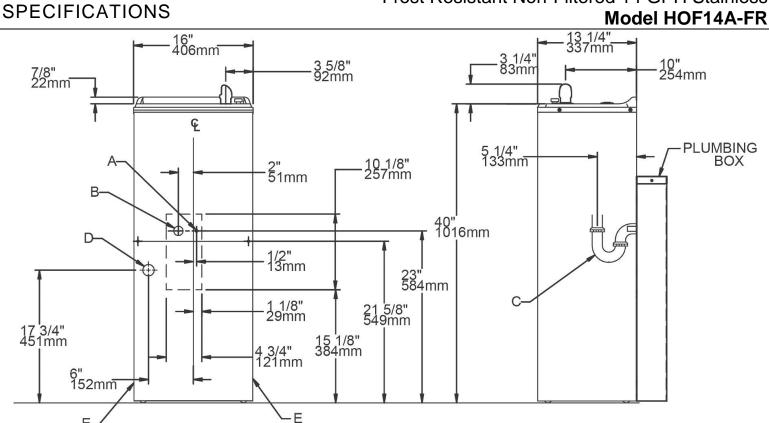
A = Recommended water supply location 3/8" (10mm) O.D. unplated copper tube connect stub 1-1/2" (38mm) out from wall - shut off valve by others. B = Recommended location for waste outlet 1-1/4" (32mm) O.D. drain. C = 1-1/4" (32mm) trap not furnished. D = Electrical outlet location with ground fault circuit interrupter (GFCI). E = Insure proper ventilation by maintaining 4" (102mm) minimum clearance from cabinet louvers to wall. F = Power cord 4' (1219mm) long.
