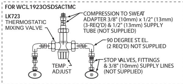
NOTE: USE TEFLON TAPE FOR ALL WATER CONNECTIONS. DO NOT USE PIPE DOPE.
