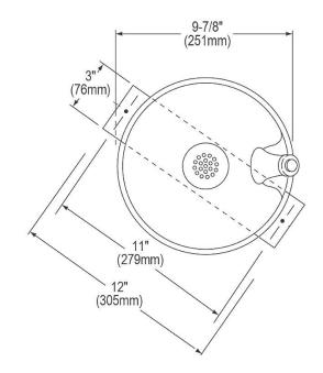
*NOTE* : Rough-in dimensions may vary 1/2" (13mm) ±. Rubber can be mounted on right or left as desired.
