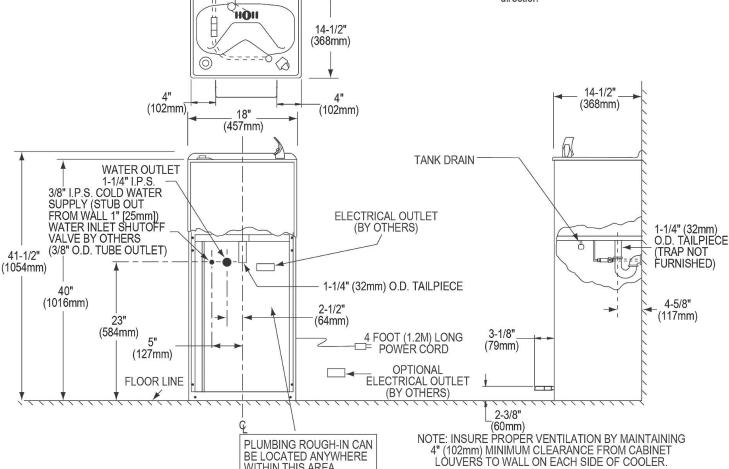
NOTE: New installations must use Ground Fault Circuit Interrupter (GFCI). It is highly recommended that the circuit be dedicated and the load protection be sized for 20 amps.
