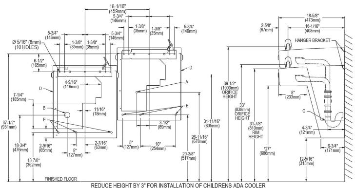
A = Recommended water supply location. Shut off valve (not furnished) to accept 3/8" O.D. unplated copper tube connect. Up to 3" (76mm) maximum out from wall.
