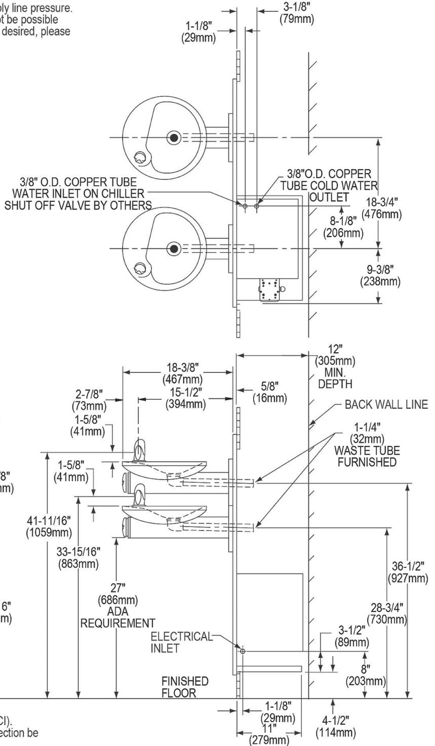
NOTE: New installations must use Ground Fault Circuit Interrupter (GFCI). It is highly recommended that the circuit be dedicated and the load protection be sized for 20 amps.
