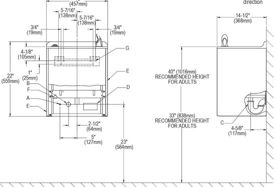
A = Recommended water supply location 3/8" O.D. unplated copper tube connect stub 1-1/2" (38mm) out from wall shut off by others.
