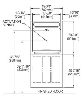
Note: New Installations Must Use Ground Fault Circuit Interrupter (GFCI). It is highly recommended that the circuit be dedicated and the load protection be sized for 20 amps.
