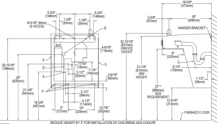
A = Recommended water supply location. Shut iff valve (not furnished) to accept 3/8" O.D. unplated copper tube. 3" (76mm) maximum out from wall.
